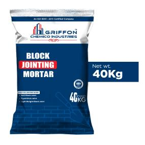
Griffon Block Joining mortar is a factory prepared blend of carefully selected raw materials, Portland cement, graded aggregates and polymers. It is suitable to use with water to produce high strength thixotropic mortar, ideal for laying aerated light weight concrete, fly ash bricks, cement hollow blocks, cellular concrete blocks or smoothing over the block work surface in layers of up to 12mm thickness.
